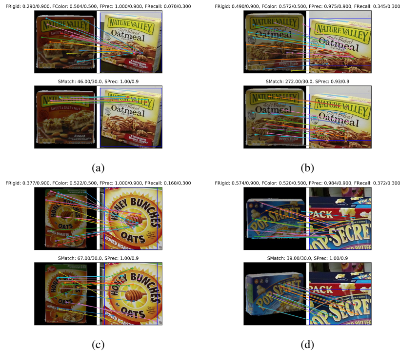
Figure 7: False detections which are incorrectly retained by SIFTVERIFY. In each image, top: FLOWVERIFY, bottom: SIFTVERIFY.
