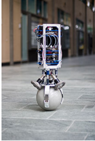
Figure 4: Image of the Ballbot used in the experiments. Ballbot is a torque-controlled, omnidirectional robot which balances on a ball through three omni-wheels.
