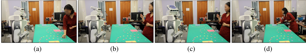
Figure 9: Real-world experiment flow: the participant a) selects the object to demonstrate, b) picks it up and shows it to the PR2, c) observes the PR2’s gaze feedback, and d) places the object in the correct bin.
