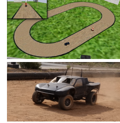
Figure 4: Top: The autonomous driving simulation environment. Bottom: The 1/5 scale AutoRally vehicle with onboard cameras used for the experiments.
