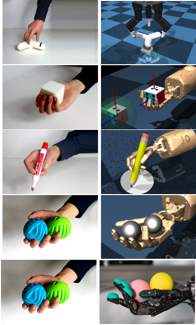
Figure 2: Task suite of simulated and real-world dexterous manipulation: valve rotation, in-hand reorientation, handwriting, and manipulating Baoding balls.
