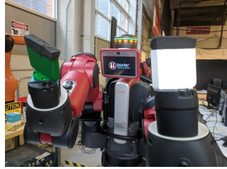
Figure 9: Close-up of compliant pushing end effectors.
