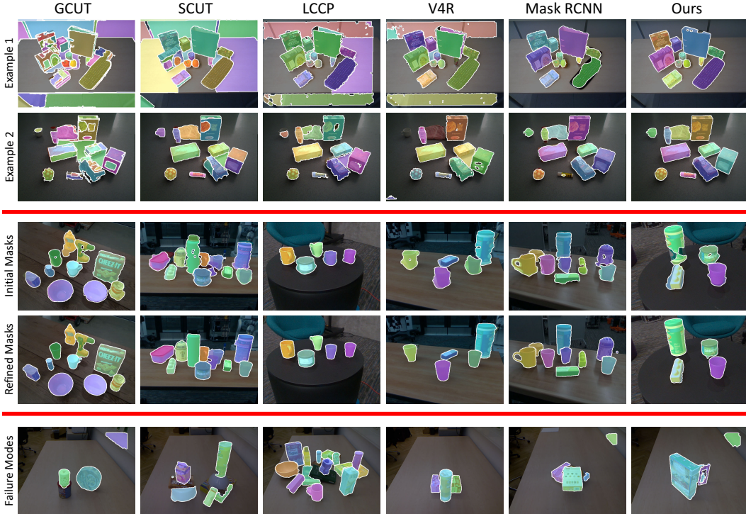
Figure 4: Qualitative results. (Top) Comparison on OCID [10]. (Middle) Mask refinements on images taken from our lab. (Bottom) Failure modes on OSD [11].
