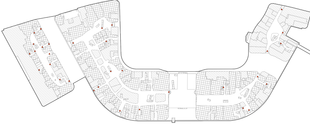
Figure 1: Sensors in first floor
