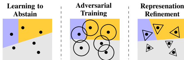
Figure 1. Illustration of the three key components used in our work. Each point represents a sample, \square is a region where model abstains from making predictions, \square and \square are regions of model prediction, \circ is the space of valid modifications for a given sample, and \triangleright is the learned (reduced) space of valid modifications.
