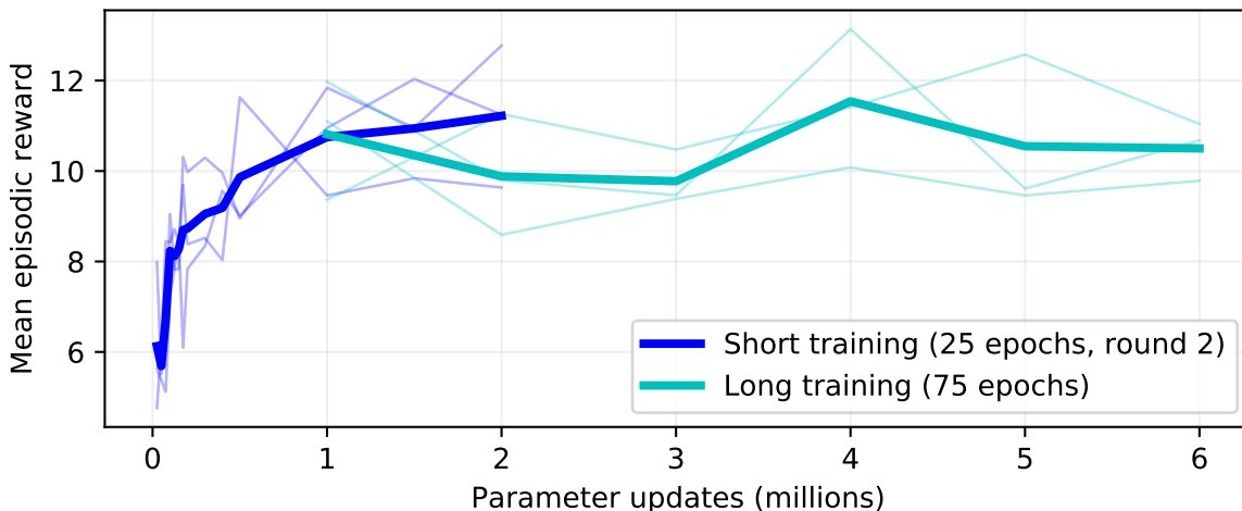
Figure 3: Learning curves of six different training runs with the round 2 submission code, three for shorter and three for longer training. Each evaluation point is an average over 200 games (standard variance in [10, 16] for agents after million updates). The first evaluation is after 25000 updates. Solid line is mean over the three runs, with individual runs shown in transparent lines. The performance of an agent can be significantly lower or higher, depending on when the training is stopped.
