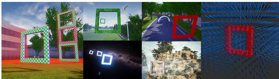
Figure 3: Sample features from our framework: Left - Environment ground truth via voxel grid, Right - Signed Distance Field gradient visualization for a gate, Middle - Examples of Domain Randomization.
