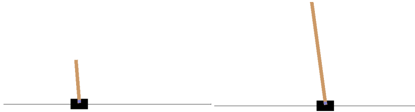
Figure 1. Illustration of the change in the dynamics for the CartPole problem. (Left) Pole’s length is 0.5m in the source environment and (Right) Pole’s length changed to 3m in the target environment.
