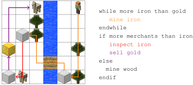
Figure 5. Example of instructions and environment state in the Minecraft-inspired domain. Correct execution begins at the first line with evaluation of the while condition, which evaluates to true because there is more iron than gold . To perform the mine iron subtask, the agent must navigate to an iron resource (the orange arrow) and perform a mine action. This removes the iron resource from the environment but the while condition still evaluates to true because there is still more iron than gold. After mining a second iron resource (second orange arrow), the numbers of iron and gold resources are equal and the while condition evaluates to false. At this point, the number of merchants in the environment (depicted as llamas) exceeds the number of iron resources and the if condition evaluates to true. The agent must then execute inspect iron and sell gold but must skip the mine wood subtask. To execute sell gold the agent must navigate to a gold resource and mine it (first violet arrow), navigate to a merchant, and then sell the gold (second violet arrow), terminating the episode with a reward of 1.
