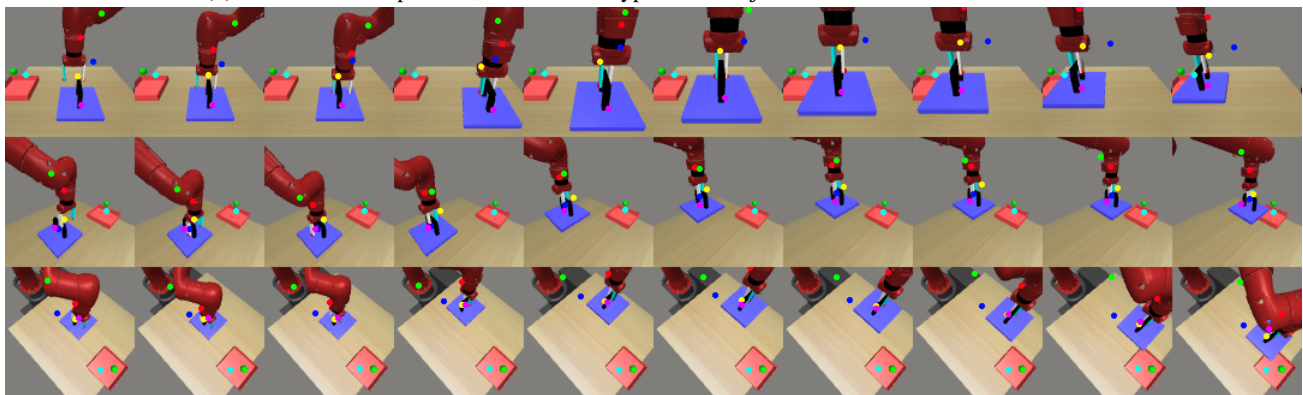
(c) In box closing, the learned keypoints track the cover, the end effector and the box
