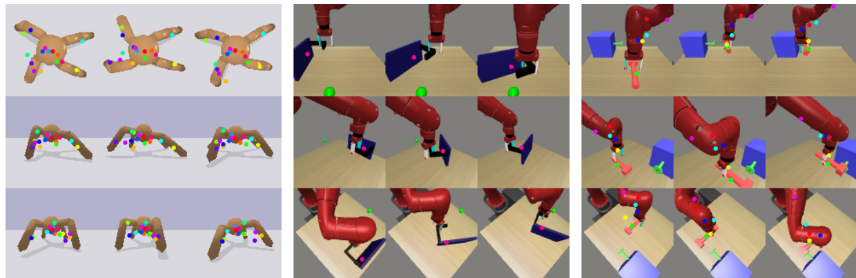
Figure 7. Visualization of the learned keypoints on colorless ant (left), metaworld close door (middle), metaworld hammer (right) environments. For the two metaworld environments, we filter keypoints with a threshold on learned keypoint attention. In colorless ant, the keypoints consistently track the limbs. In door the pink point with highest confidence tracks the movement of the door consistently. In hammer, the green point tracks hammer, while other points tracks the end-effector and sections of the arm respectively.
