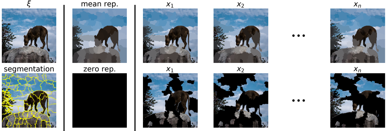
Figure 2. Sampling procedure of LIME for images. The image to explain, \xi , is first split into d superpixels ( lower left corner , here d = 72 ). A replacement image \bar{\xi} is computed, which is by default the mean of \xi on each superpixel ( top row ), see Eq. (1). This replacement image can also be filled uniformly with a pre-determined color ( bottom row : replacement with the color black). Then, for each new generated example x_i with 1 \leq i \leq n , the superpixels are randomly switched depending on the throw of d independent Bernoulli random variables with parameter 1/2 . Thus LIME creates n new images where key parts of \xi disappear at random.
