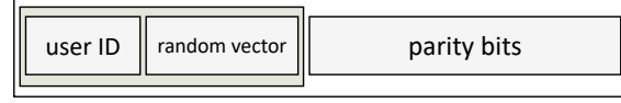
Figure 1: Structure of secret codewords. The secret vector of each user is the concatenation of a message vector and the corresponding parity bits obtained using an error-correcting code (ECC). The message vector itself is composed of two parts, 1) a unique binary vector representing the user ID, and 2) a random binary vector chosen by the user. This construction provides the following properties: i) vectors are unique because the user ID is unique, ii) vectors are secret because the random vector is not known to other users or the server, and iii) vectors are guaranteed to be maximally separated due to the use of ECC algorithms.
