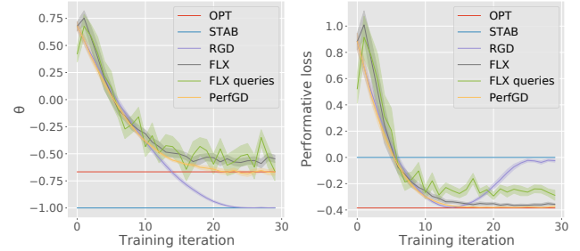
Figure 1. Results for a modified version of the toy example introduced in Section 2.2. OPT denotes the performatively optimal point \theta_{\text{OPT}} , and STAB denotes the performatively stable point \theta_{\text{STAB}} . Since the mean is nonlinear in \theta , estimating df/d\theta with finite differences is more challenging. In spite of this, PerfGD still converges to the optimal point. FLX also finds a decent point, though its query points are worse than those of PerfGD.
