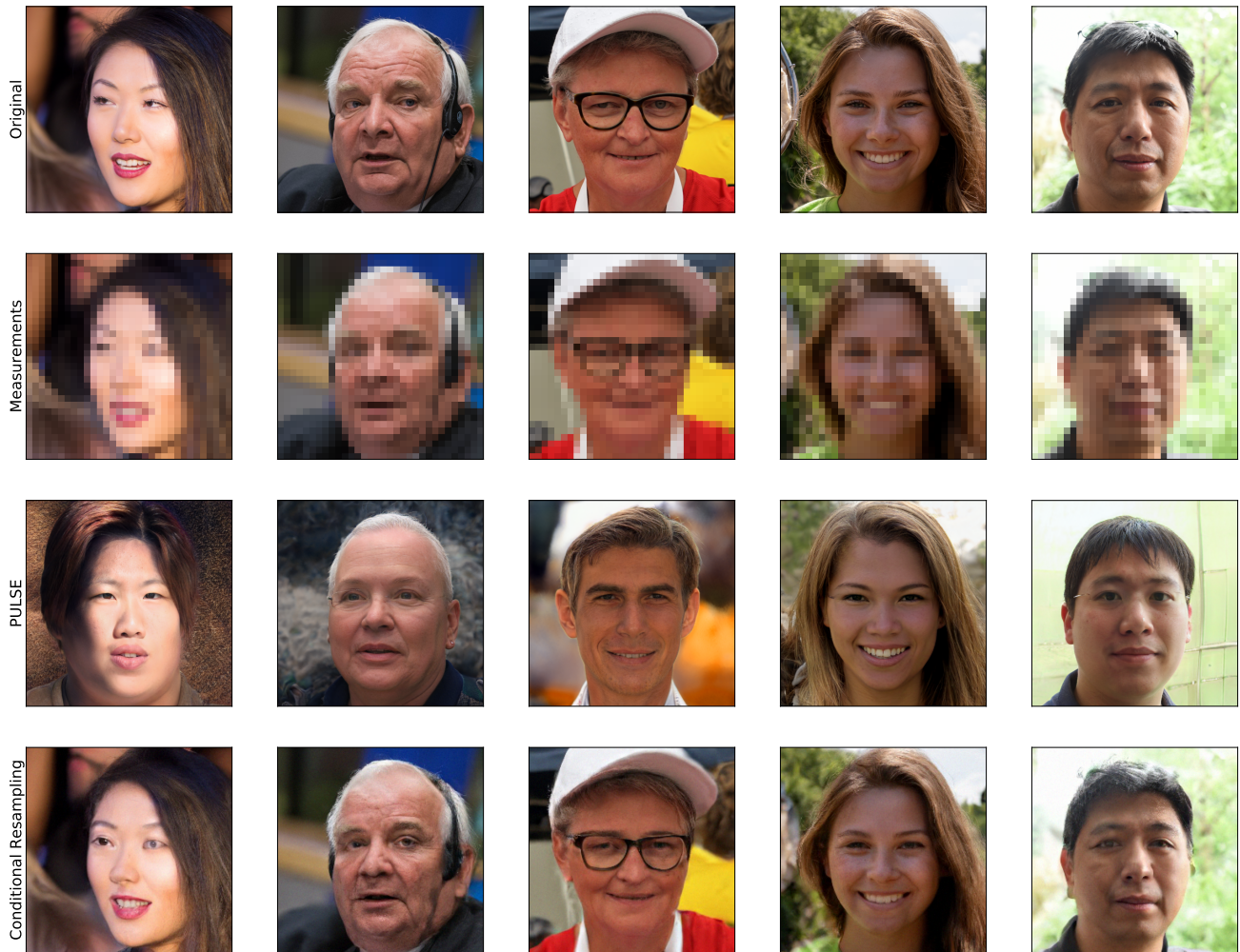
Figure 5. Super-resolution reconstructions on faces 69000-69004 from the FFHQ dataset. The top row shows original images, the second row shows what the algorithms observe: blurry measurements after downsampling by 32\times in each dimension. The third row shows reconstructions by PULSE, and the last row shows reconstructions by Posterior Sampling via Langevin dynamics, the algorithm we are advocating for.
