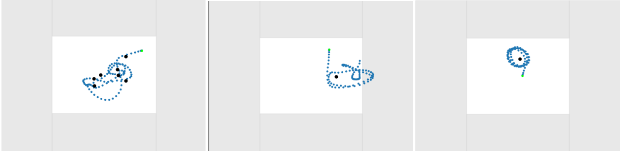
Figure 13. BC: The failure cases come from one of the demonstrations having the same behavior of circling the trash without picking it up. Since BC is only incentivized to exactly mimic the actions in demonstration states, it is unable to navigate ambiguities in the demos.
