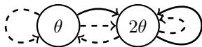
Figure 1. A simple two State MDP. The solid lines depict the (deterministic) target policy \pi(\text{right}|\cdot) = 1 . Dashed lines denote the (more exploratory) behavior policy \mu . The behavior policy selects any of the actions with equal probability \mu(\text{right}|\cdot) = \mu(\text{left}|\cdot) = 0.5 , in all states. The rewards are zero everywhere.
