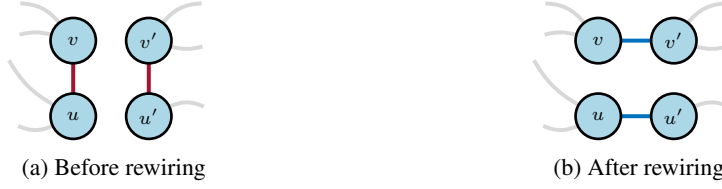
Figure S1. In the rewiring operation the red edges are deleted and the blue edges are added. The degree of each node remains the same.
