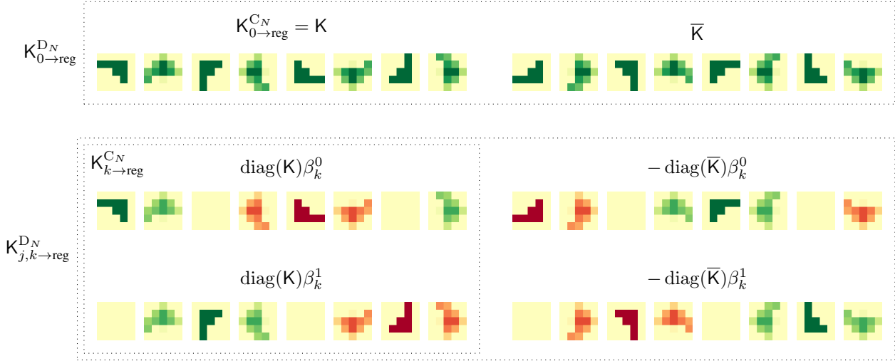
Figure 3. Visualization of FILTRA filter examples. Based on a same weight kernel K , we generate filters K_{0 \rightarrow \text{reg}}^{C_N} , K_{0 \rightarrow \text{reg}}^{D_N} , K_{k \rightarrow \text{reg}}^{C_N} and K_{j, k \rightarrow \text{reg}}^{D_N} . In this example we set j = 1 , k = 1 , N = 8 . The two-columns of matrix \beta_k is splitted as \beta_k^0 and \beta_k^1 for visualization. Red, light yellow and green denotes negative, 0 and positive values, respectively. Please view this figure in color.
