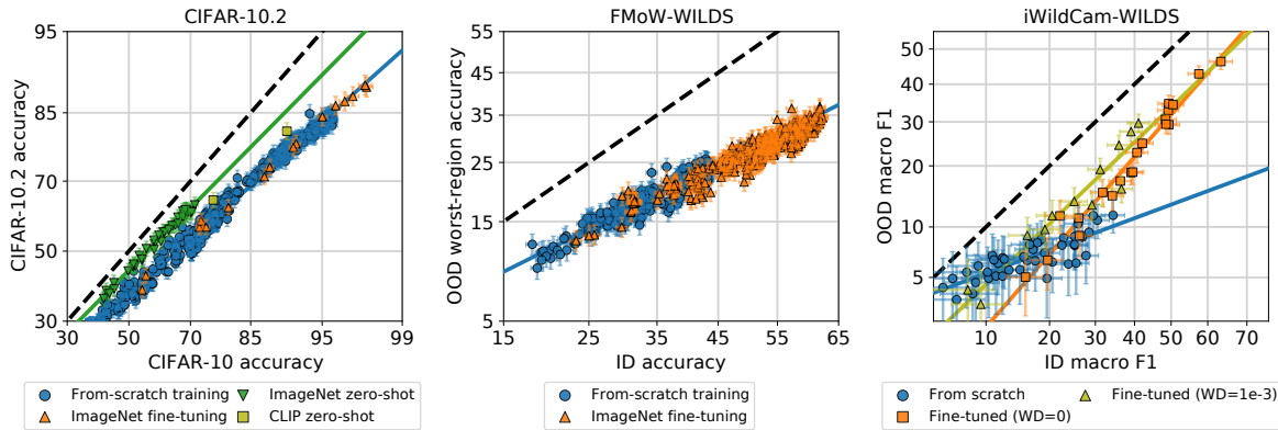
Figure 4. The effect of pre-training with additional data on CIFAR-10.2 (left), FMoW-WILDS (middle), and iWildCam-WILDS (right). On CIFAR-10.2 and FMoW-WILDS, fine-tuning pretrained models moves the models along the predicted ID-OOD line. However, on CIFAR-10.2, zero-shot prediction using pretrained models deviates from this line. On iWildCam-WILDS, fine-tuning pretrained models changes the ID-OOD relationship observed for models trained from scratch. Moreover, the weight decay hyperparameter affects the ID-OOD relationship in fine-tuned models.
