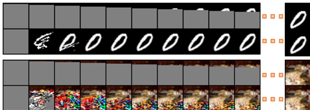
Figure 2. Feedforward (1st & 3rd rows) vs. Jacobi (2nd & 4th rows) sampling for PixelCNN++ on MNIST (top 2 rows) and CIFAR-10 (bottom 2 rows). Each column corresponds to the same number of updates. We show the first few intermediate samples on the left and the final image samples on the rightmost.
