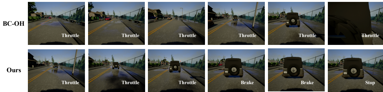
Figure 5. An example test scenario from CARLA navigated by a BC-OH policy (top) and ours (bottom). Frames displayed in sequence from left to right. Actions (“Throttle”/“Brake”) are overlaid on the frames.
