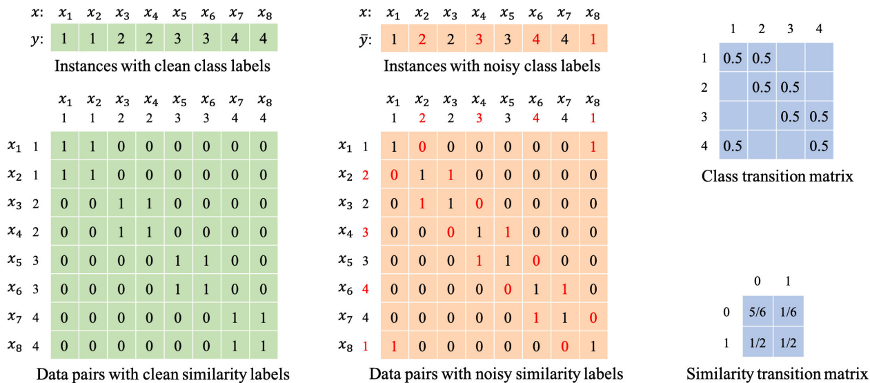
Figure 1. An illustration of the transformation from class labels to similarity labels. Note that \bar{y} stands for the noisy class label and y for the latent clean class label. The labels marked in red are incorrect. If we assume the class label noise is generated according to the transition matrix presented in the upper part of the right column, it can be calculated that the noise rate for the noisy class labels is 0.5 while the noise rate for the noisy similarity labels is 0.25. Note that the transition matrix for similarity labels can be calculated by exploiting the class transition matrix as in Theorem 1.
