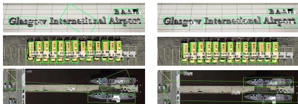
Figure 1. Comparison of the detection results between Smooth L1 loss-based (left) and the proposed GWD-based (right) detector.
