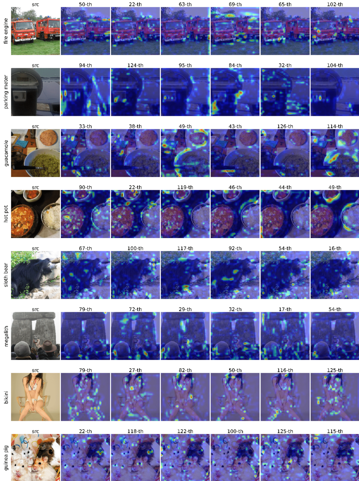
Figure 3. Visualization of attention weights generated by our method (from the last block in “ model.layer2 ”). Each row represents one image with its correspondence attention weights. We randomly select different (shown as “X”-th) channels from our 3-D weights to show.
