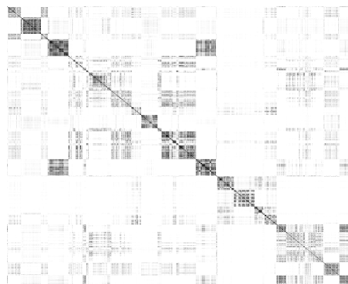
Figure 3: Class sorted kernel matrix for the weighted average of the DTW and call shape parameters representations.
