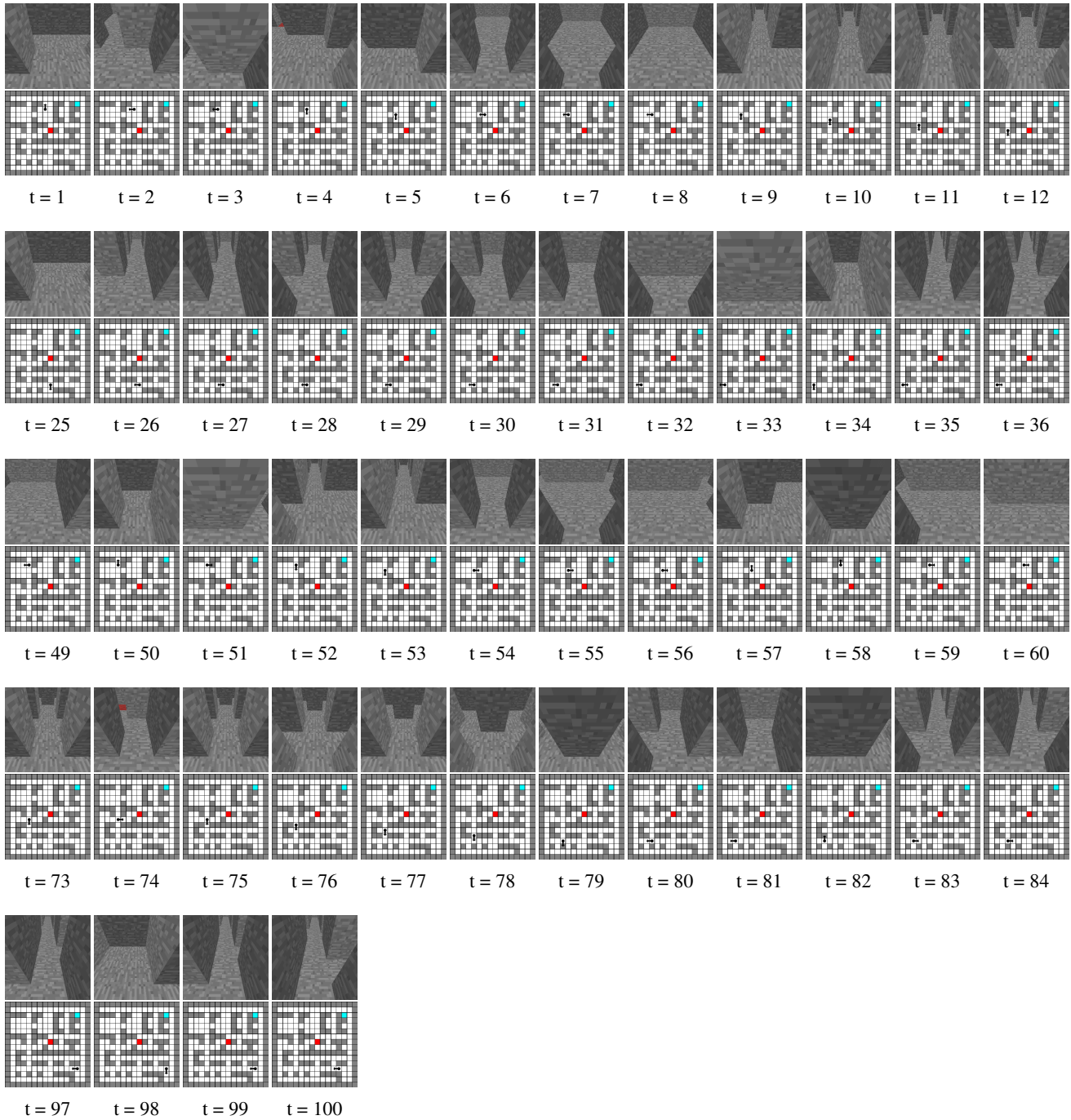
Figure 7. FRMQN’s play in an unseen and larger random maze with Single Goal task. Even though the agent explores the entire map in a reasonable way, it fails to find the blue block within 100 steps. This can occur occasionally, especially when the map is quite large and intrinsically complex (e.g., contains many walls giving rise to deep partial observability).
