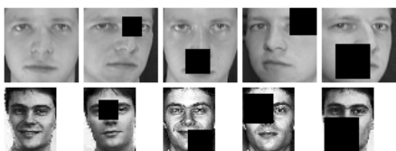
Figure 3: Sample images from ORL (up) and FERET (bottom) databases with occlusion patch sizes as 0-by-0, 16-by-16, 20-by-20, 24-by-24, and 28-by-28 pixels respectively.
