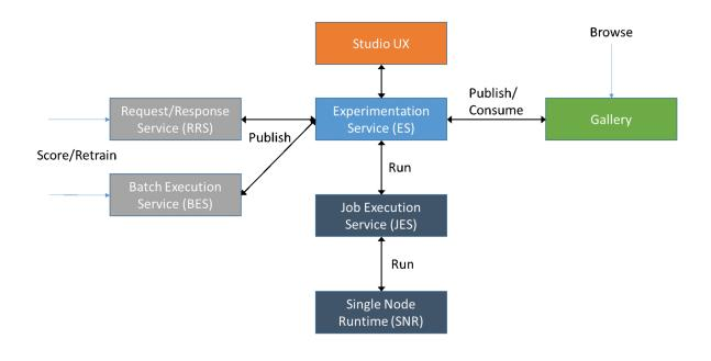
Figure 2: Component services of AzureML
