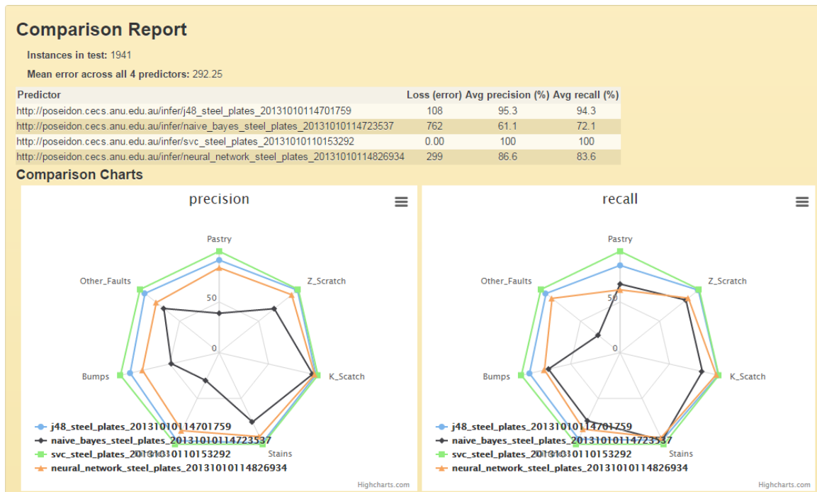
Figure 4: Part of the output from the demonstration JavaScript client’s classifier comparison tool. Its inputs are URIs for the testing data attributes and predictors to compare
