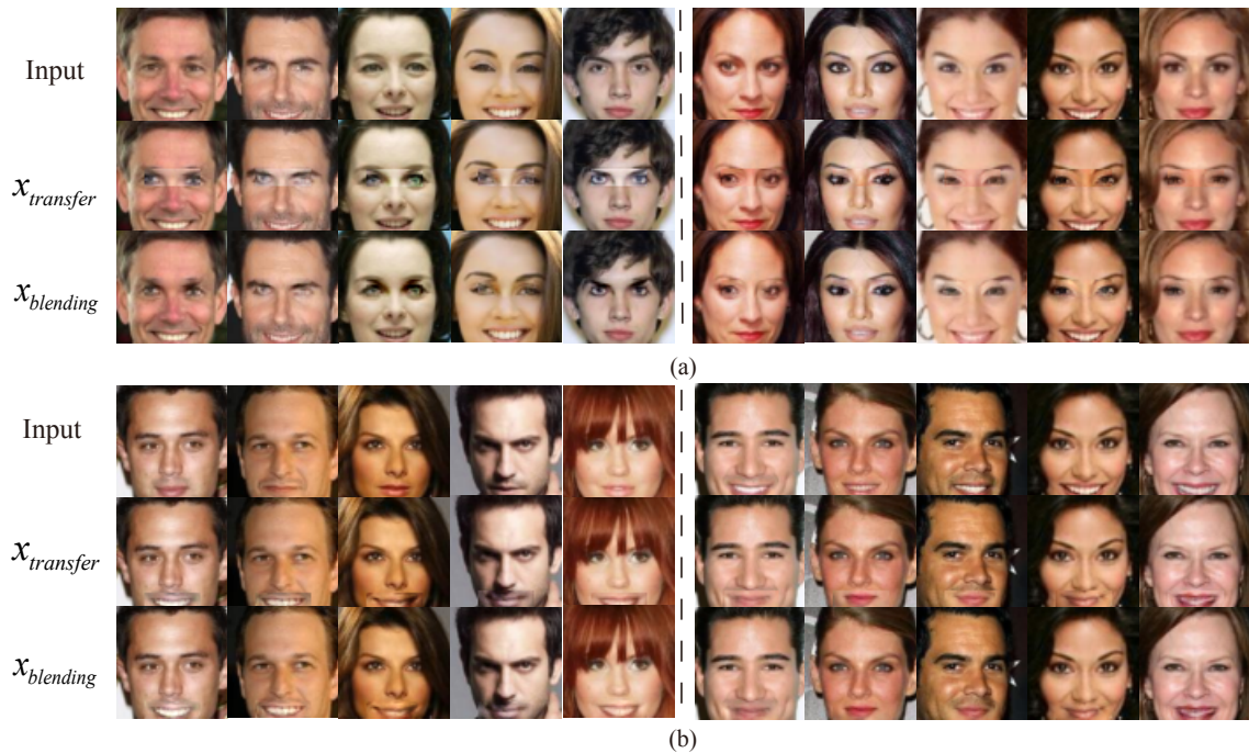
Figure 8: Facial image Semantic Transformation for local regions by changing latent code c_2 . (a) We show that LST-GAN can transform the semantic features of the eye region. In the left images, The faces are transformed into faces with larger eyes. In the right images, the faces are transformed into faces with smaller eyes. (b) We show LST-GAN can transform a face between with a closed mouth into one with an open mouth. Poisson blending is used as the final transformation result x_{blending} to preserving the same intensities of the surrounding pixels.
