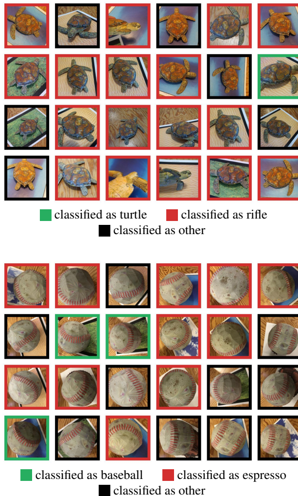
Figure 5. Random sample of photographs of the two 3D-printed adversarial objects. The 3D-printed adversarial objects are strongly adversarial over a wide distribution of viewpoints.
