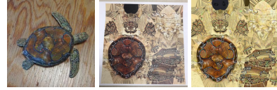
Figure 7. A side-by-side comparison of a 3D-printed model (left) along with a printout of the corresponding texture, printed on a standard laser color printer (center) and the original digital texture (right), showing significant error in color accuracy in printing.
