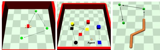
Figure 3. From left to right (1) the wheeled locomotion environment with the waypoints depicted in green (2) the object manipulation environment with different objects (blocks and cylinders) and their correspondingly colored goals (squares) (3) the swimmer navigation task with the first 3 waypoints depicted in green.
