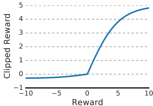
Figure D.1. Optimistic Asymmetric Clipping - 0.3 \cdot \min(\tanh(\text{reward}), 0) + 5.0 \cdot \max(\tanh(\text{reward}), 0)
