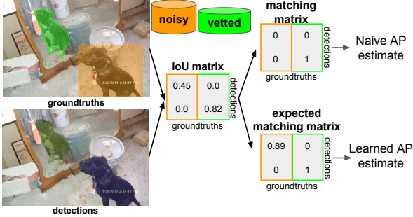
Figure 3. Standard instance segmentation benchmarks ignore unvetted data (top pathway) when computing Average Precision. Our proposed estimator for this task computes an expected probability of a match for coarse bounding box annotations when vetted instance masks aren't available.
