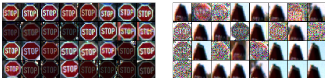
Figure 7: Example from one experiment (seed) of the 32 most normal (left) and 32 most anomalous (right) examples on GTSRB stop signs test set according to Deep SVDD anomaly scores ordered by score from top left to bottom right. The example shows that Deep SVDD detects adversarial attacks.
