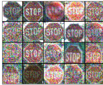
Figure 5: The 20 adversarial examples generated by using Boundary Attack.
