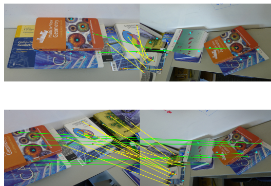
Figure 3. Two instances of matchings in Books dataset which is severely occluded. Yellow/green lines show correct/incorrect matches and isolated points show no matches.
