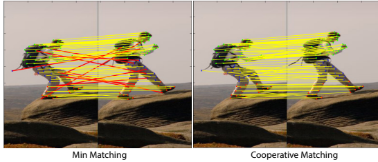
Figure 1: An illustration of cooperative matchings. The goal is to match corresponding points between the two images. On the left, bipartite matching is used and there are many mismatched points (indicated by red edges). On the right, similar points are clustered and offered a within-cluster discount via a submodular function, significantly reducing the number of mis-matched points.
