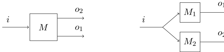
Figure 1: A Moore machine with two outputs (left) can be equivalently seen as two (potentially smaller) Moore machines with a single output each (right).
