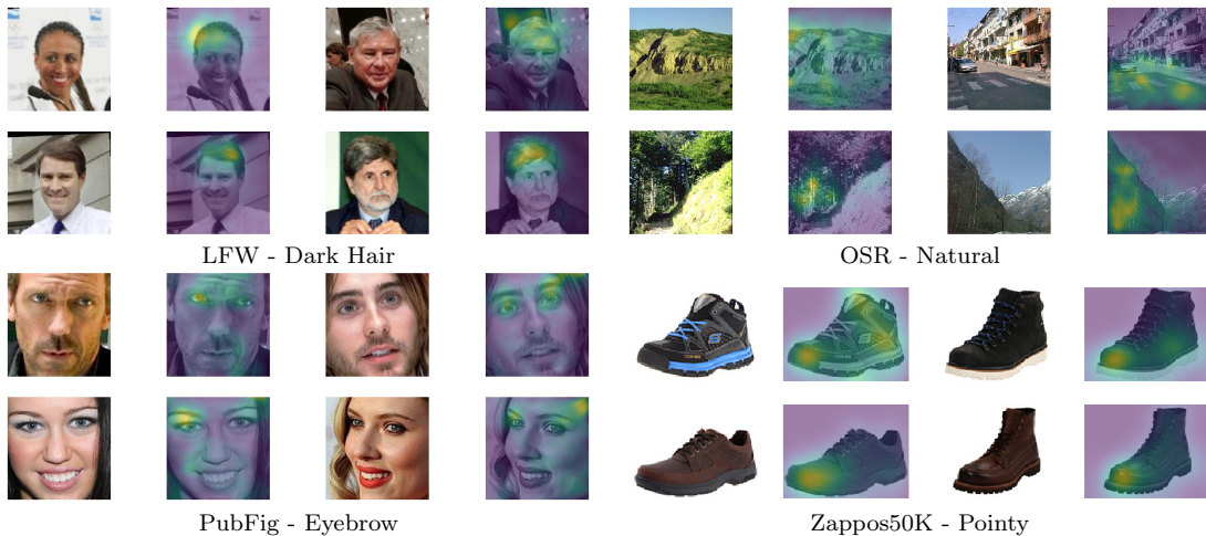
Figure 4: Saliency maps generated by our model. For each dataset, 4 test images and their overlaid saliency maps are shown (the warmer the color of the overlay image, the more salient that pixel is). As shown, our model pays attention to the relevant regions: hair for dark hair, plants and road for natural, regions around eyes for eyebrow, and toe end for pointy.
