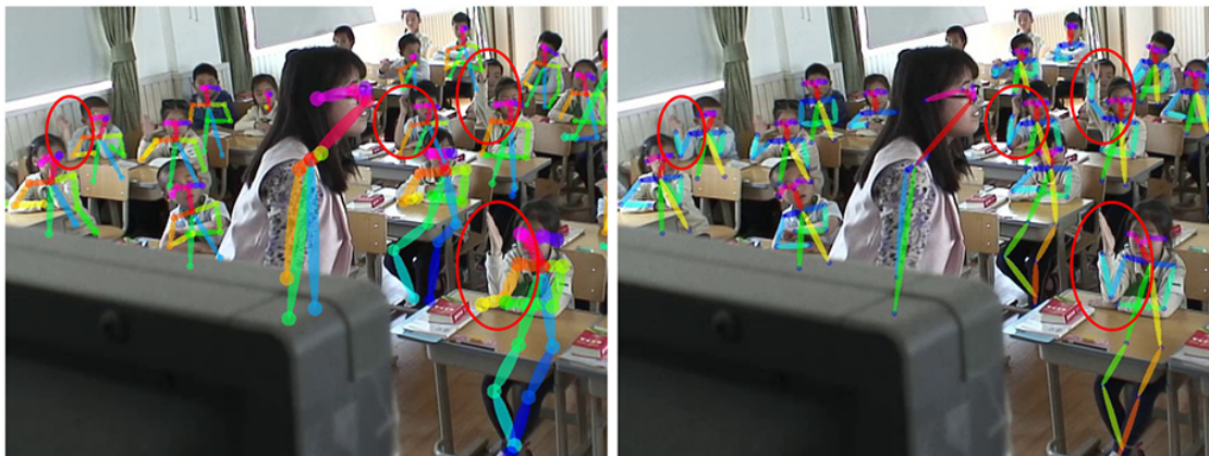
Figure 6: The left image is the result of the original method. No joint points have been detected of the raising hands. The right image is obtained by our modified method. The joints of the four raising hands are errorless.
