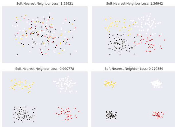
Figure 1. A set of 200 2D points is sampled from a Gaussian and labeled randomly. Then, using gradient descent on the x and y coordinates of the points, the soft nearest neighbor loss is minimized to decrease entanglement. The 4 classes become more isolated. While a direct comparison with other losses like cross-entropy is not possible for this experiment, we inspect and compare non-entangled and entangled representation spaces later in the paper.
