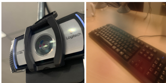
Figure 1. Illustration of our approach: (left) our adversarial sticker affixed to a camera lens; (right) view from the camera with sticker, where the keyboard is reliably classified as a computer mouse for most viewpoints and scales.
