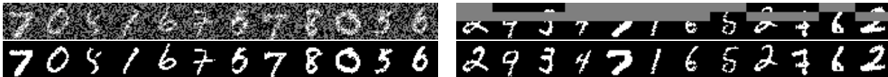
Figure 1. Random incomplete samples from the MNIST training data set, and single imputations obtained by MIWAE (trained with K = 50 importance weights, and imputed with L = 10\,000 importance weights). The MCAR data set is on the left, and the MAR data set is on the right.
