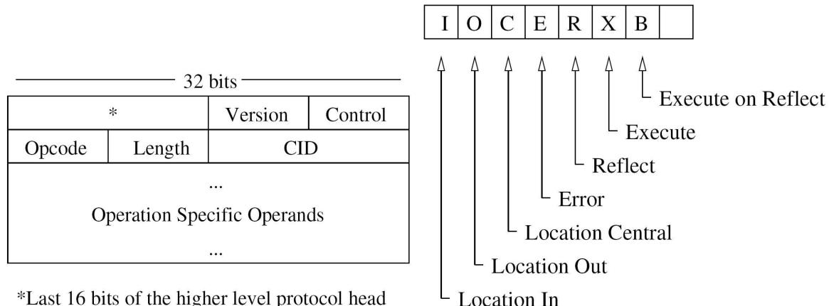
The Execute bit tells an ESP enabled system whether the packet is just "passing though" or needs to be processed.
