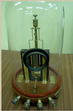
Fig. 12 – Deprez D'Arsonval's galvanometer – A suspended coil galvanometer (11)
